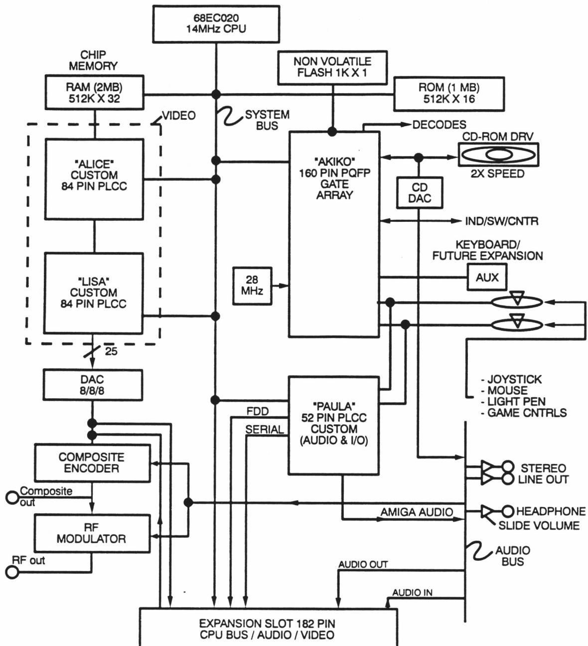
Figure 4-1. Amiga CD<sup>32</sup> Block Diagram
