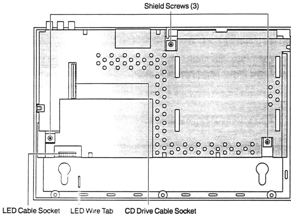
*Figure 2-2. Motherboard Shield and Cable Socket Locations*
